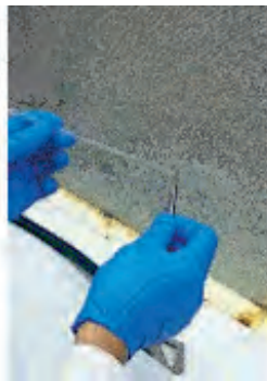
2) Pull ends apart to stretch glass.
